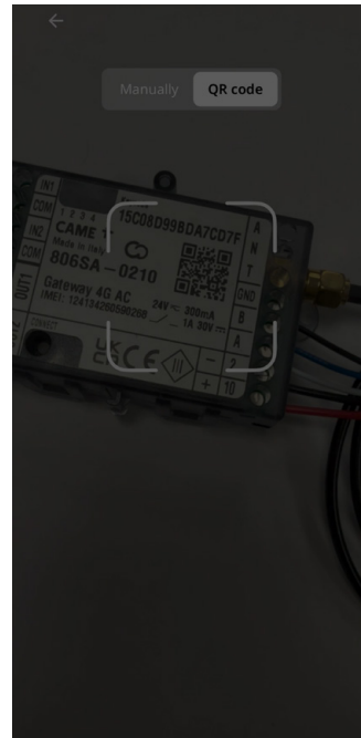
4.3 You can use the camera to scan the QR code label to automatically add the Gateway device to the Installation. Select 'QR code' to carry out this method of adding.
