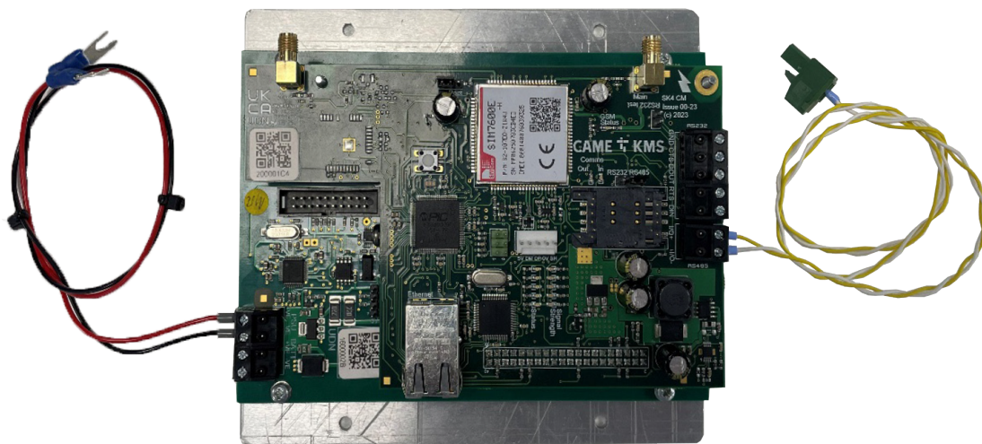
FIGURE 7.2 4G MULTI COMMS MODULE ON A BASEBOARD
