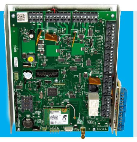
The SimpleKey 4 system controller is the central component of the latest generation of the SimpleKey platform. Incorporating a number of innovative features enabling simpler installation, expansion and management. The SimpleKey 4 system controller has a built in GPRS modem for communications and connections for controlling the first two doors. The system can be easily expanded on a door by door basis using additional SimpleKey 4 extension kits on a free topography wiring bus.
