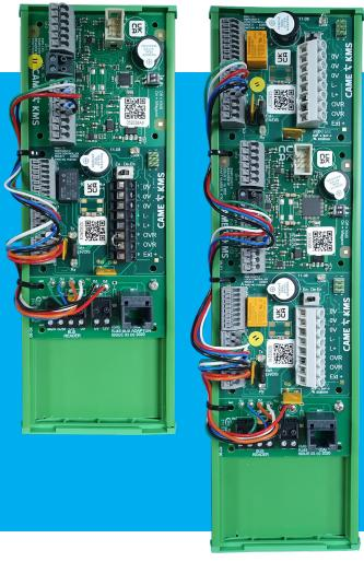
The SimpleKey 4 door extension kits allow additional doors to be controlled when connected to a SimpleKey 4 system controller. Available in one or two door versions, in a DIN rail format with simple connections to the free topography KMS Bus.
