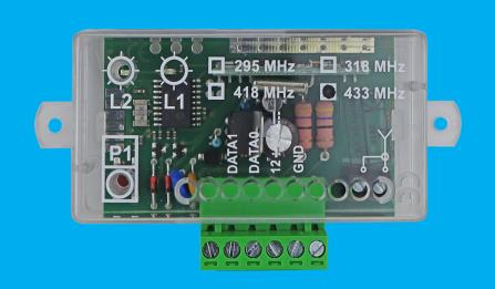
This Wiegand receiver 26 bit allows use of radio transmitters for connection to online access control systems.
