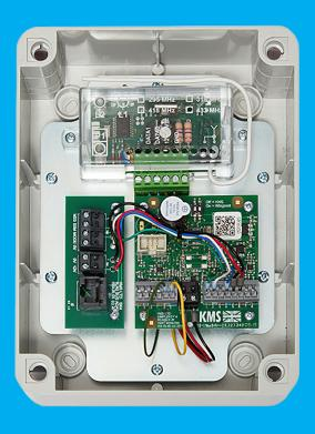
26 bit SELW-R433 Wiegand receiver allows use of radio transmitters for connection to online access control systems.
