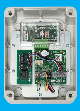
Includes Reader Interface for connectivity to SimpleKey 4 Access Control System
