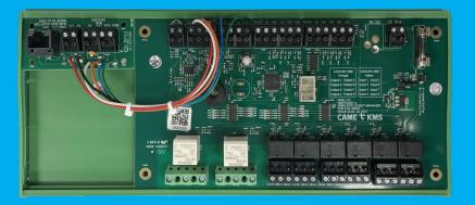
SimpleKey Event Manager (SEM) allows additional building functions to be controlled and monitored when connected to a SimpleKey system controller.
