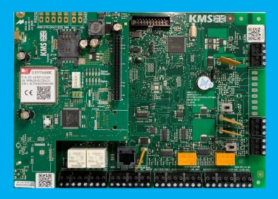
Available in three versions, 4G, IP & Multi allowing the SimpleKey System Controller to easily connect to SimpleKey Web;
