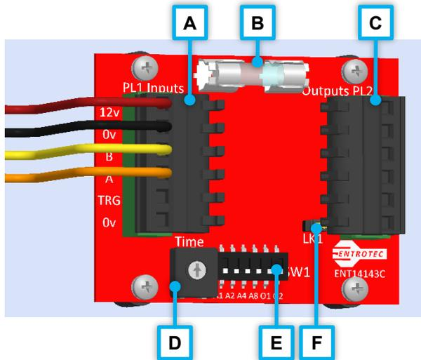
FIGURE 20 – SLR WITH FACTORY FITTED CONNECTIONS
