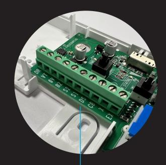
Handset wiring connector to APEX or ELITE marshalling board.
