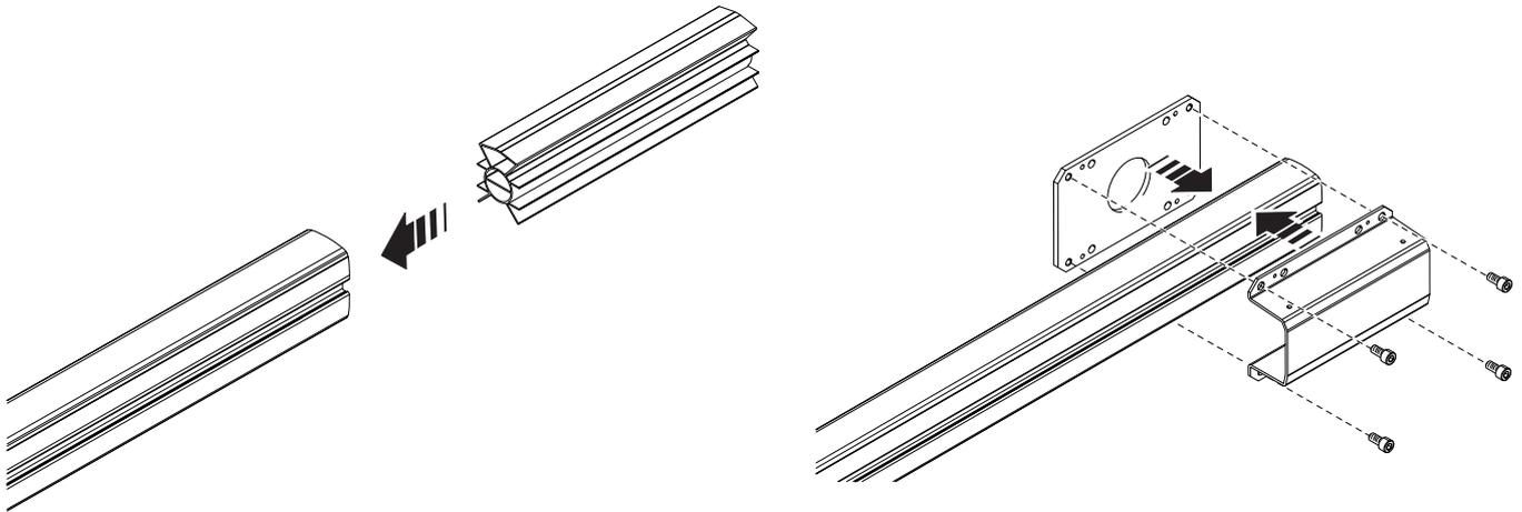
Fix the boom to the anchoring plate.
