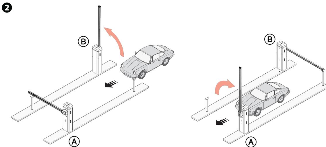
3 OPEN-CLOSE command (2-7) on barrier A or B for emergency opening
